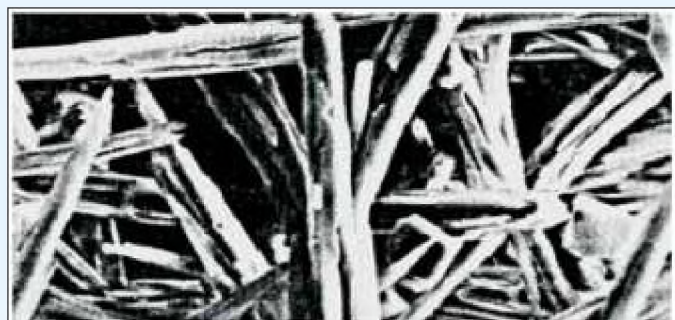
Picture 11: Lime dust deposits
